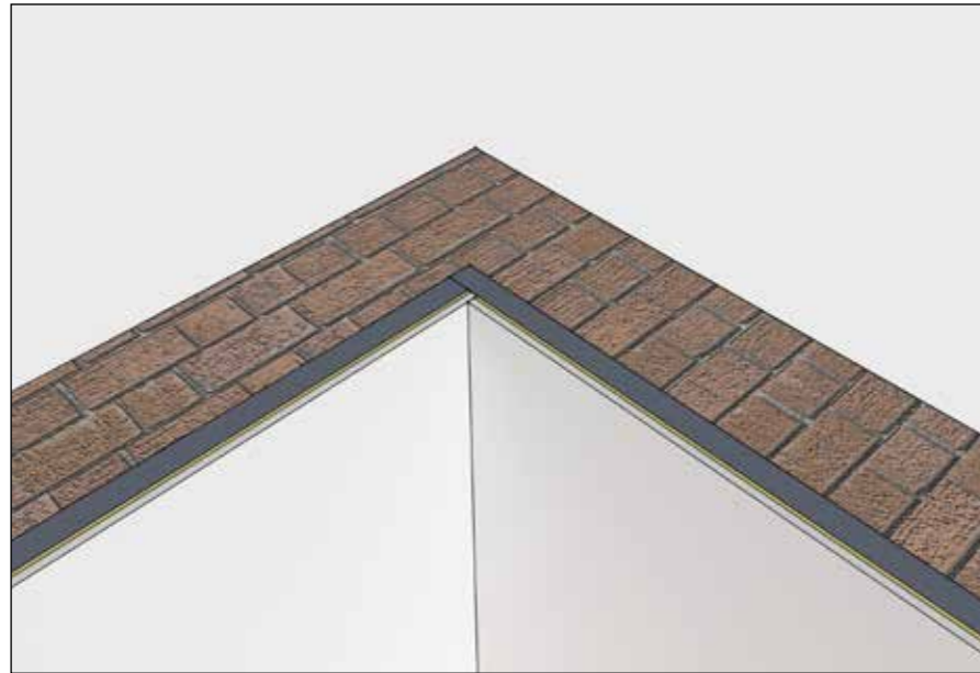
Fig. 6 Internal angle joint in Spacetherm WL
