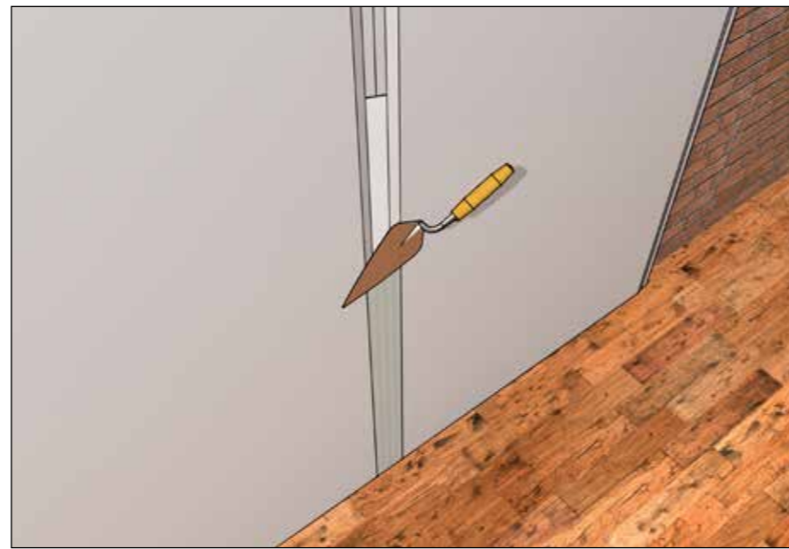
Fig. 8 Taping and Filling Joints in Spacetherm Directfix
