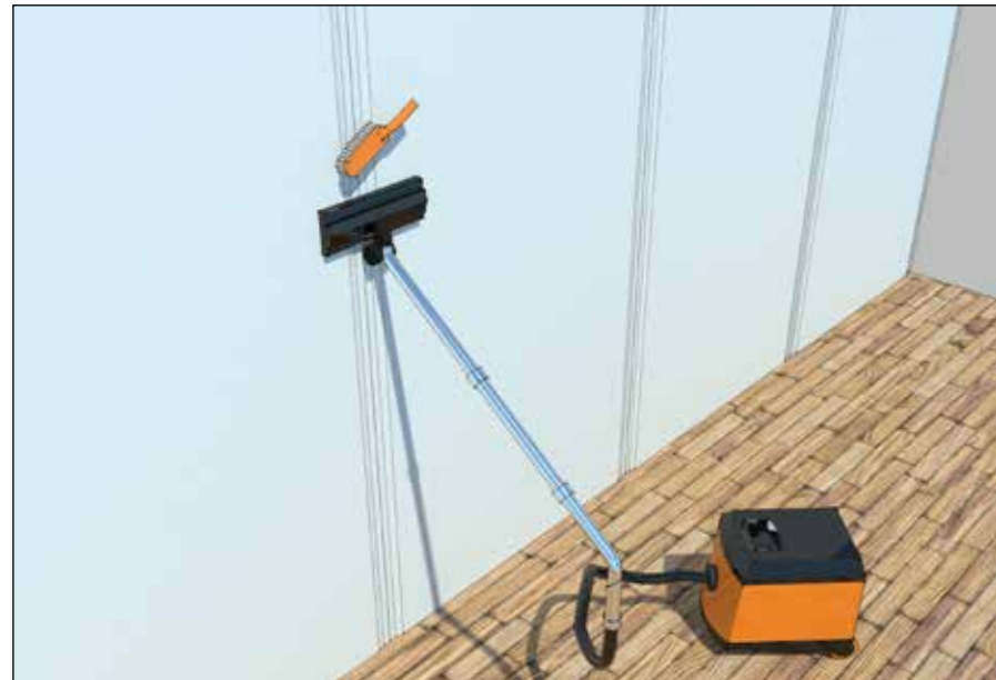
Fig. 7 Preparing Spacetherm Multi Surface for Jointing
