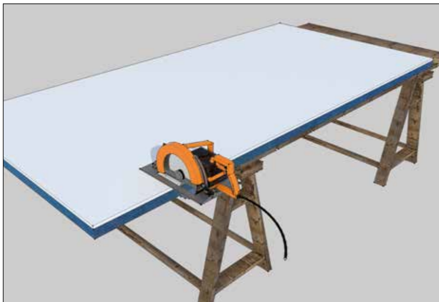
Fig. 2 Cutting Spacetherm Multi Boards
