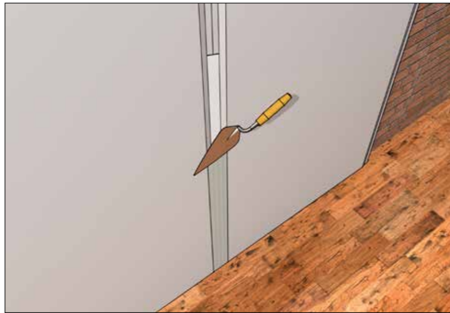
Fig. 8 Taping and Filling Joints in Spacetherm Wallboard / A2 Wallboard
