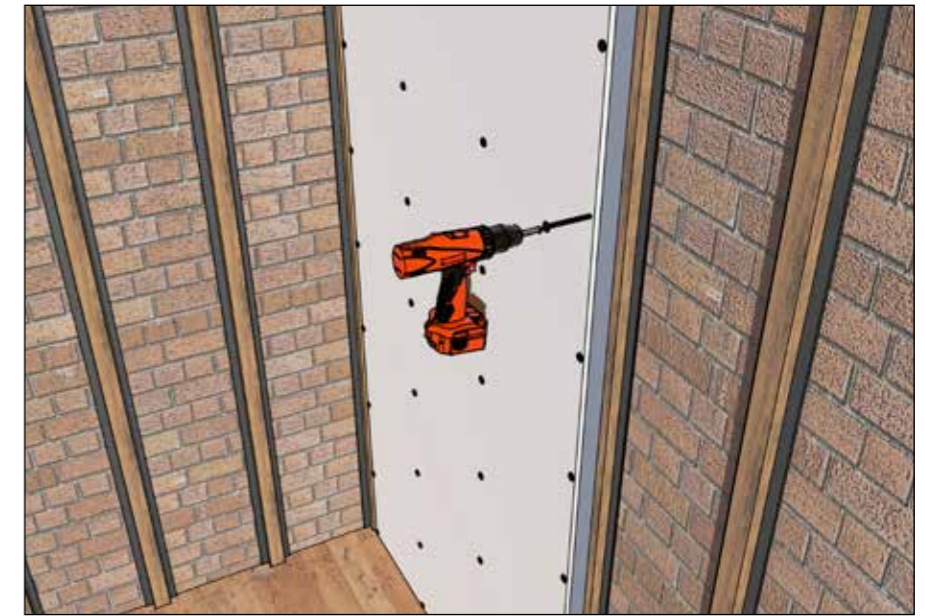
Fig. 4 Fixing Spacetherm Wallboard / A2 Wallboard to Timber Straps
