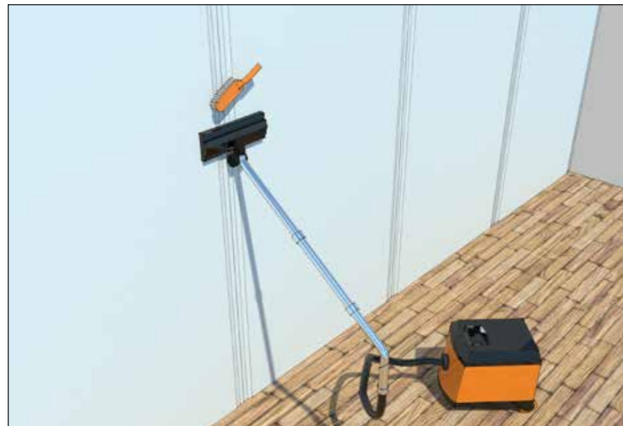
Fig. 7 Preparing Spacetherm Multi / A2 Multi Surface for Jointing
