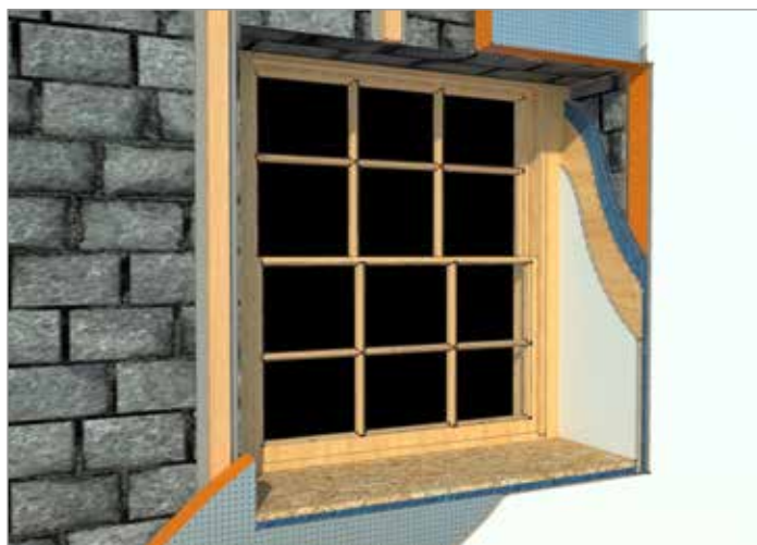
Image showing Spacetherm WRB applied internally to a reveal on an existing external wall structure.
