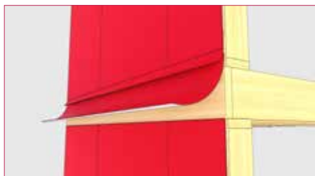
Floor Junction on installation
