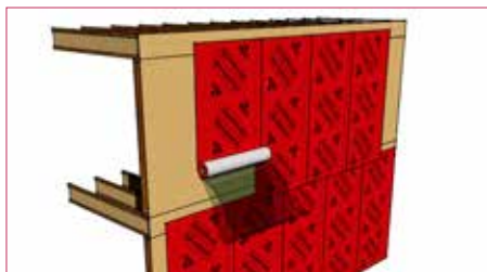
Vertical over sheathing
