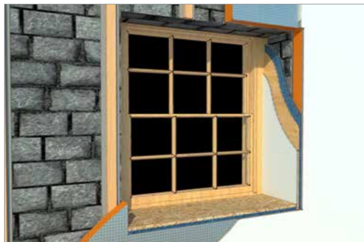
Image showing Spacetherm WRB applied internally to a reveal on an existing external wall structure.
