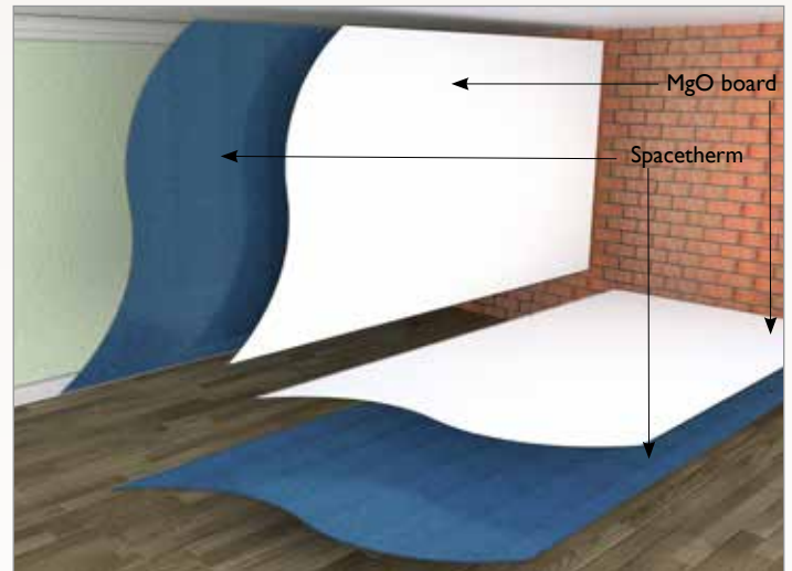
Image showing Spacetherm Multi applied internally to an existing external wall structure.
