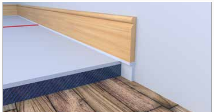
Fig 1 - Spacetherm Multi skirting detail
