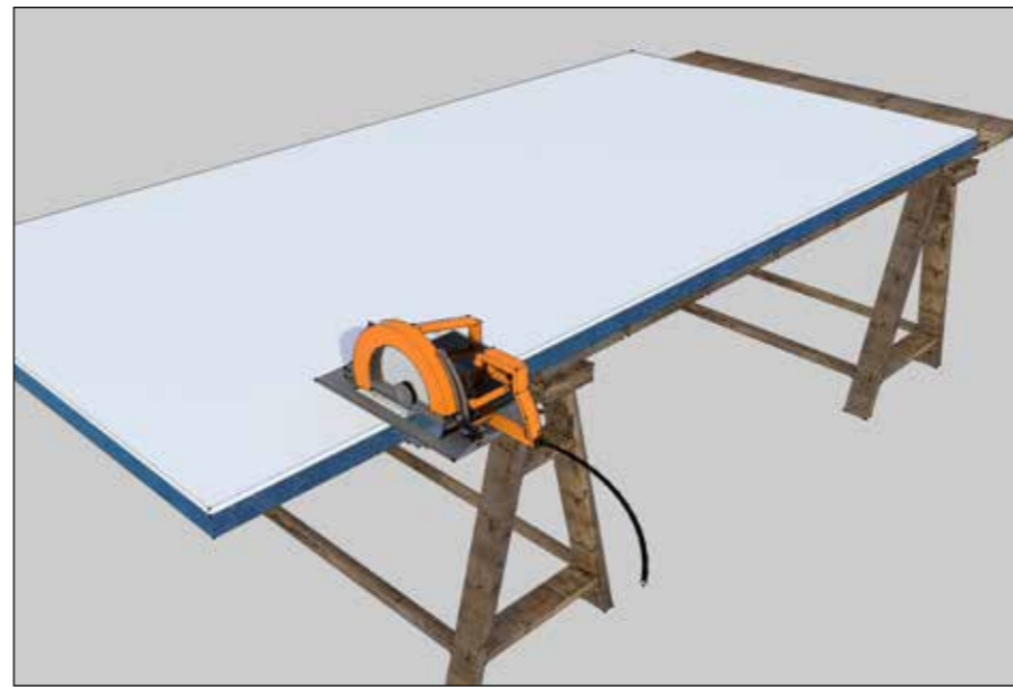
Fig. 2 Cutting Spacetherm Multi Boards
