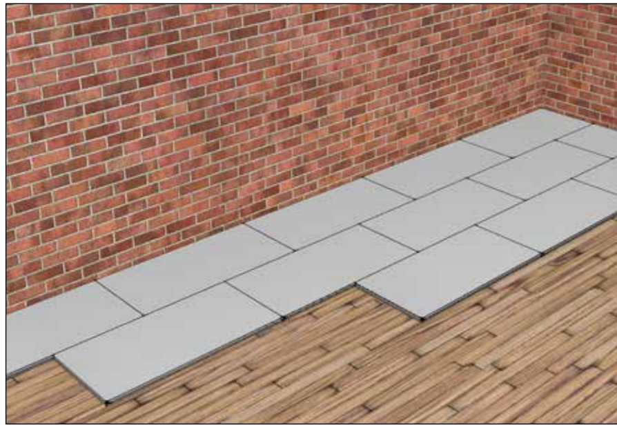
Fig. 4 Board installation pattern for Spacetherm Multi
